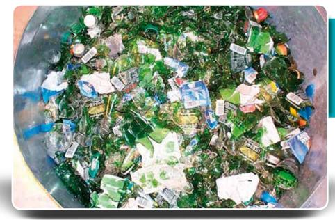
Using a compactor to crush glass into 'cullet' will save space, reduce the number of vehicle collections and reduce noise at collection times
